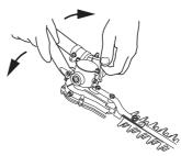
Grasp the handle on the angle stop, adjust to the desired angle and then tighten the knob.
